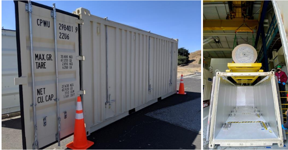
Figure 2. Camera Shipping Container (Container 1A). Inside view on the right shows the insulation on the walls, securing hardware on the floor, and open top for a test lift of a mass simulator for the Camera.
