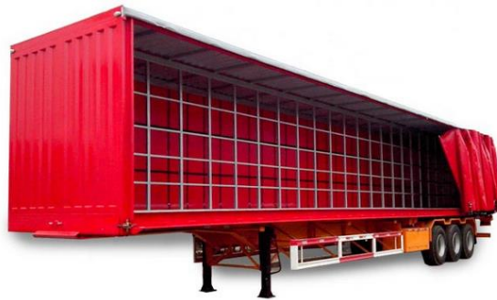
Figure 5. Side load trailer for break bulk cargo with rolling tarps on the side.
